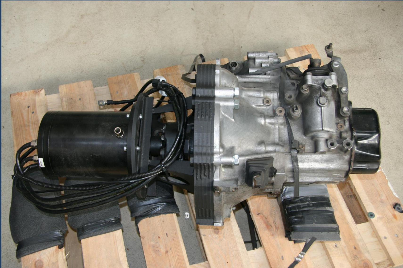
Pic.6. Electric motor, clutch and gearbox ready to assembly.
