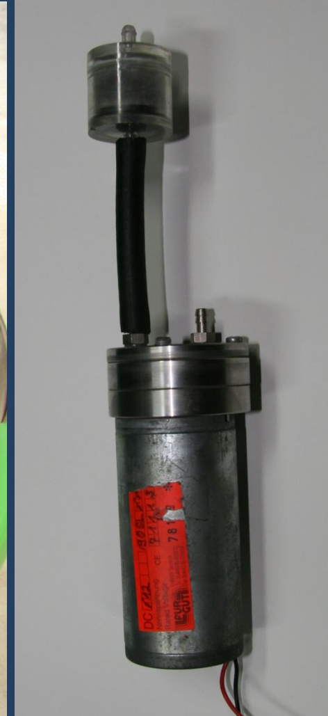
Pic.12. Break system; the vacuum pump and battery (brake pedal inside the cabin).
