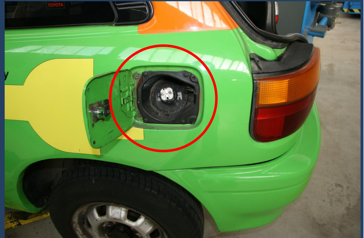
Pic.15. Battery management system (BMS) and charger socket.
